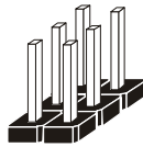
Jumper Block looks like this
