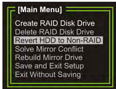
Figure D-14: Revert HDD to non-RAID
