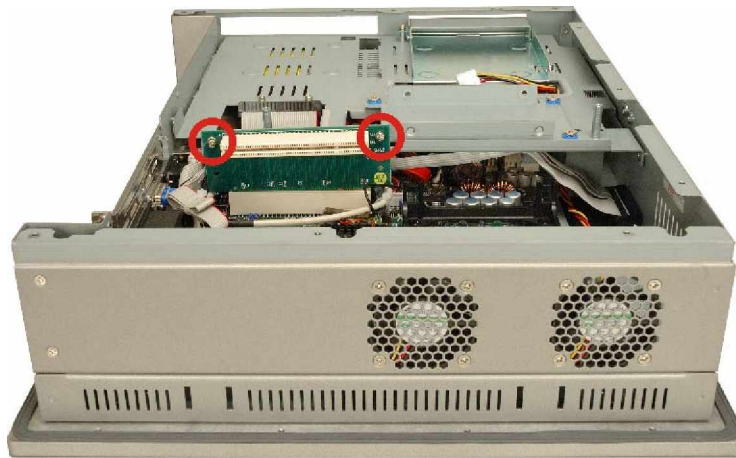
Figure 4-7: Elevated Platform Retention Screws (PCI Riser Card)
