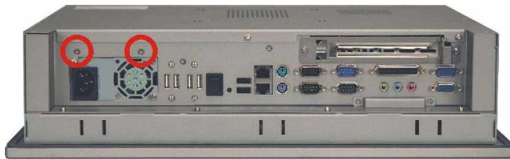
Figure 3-6: CD Drive Retention Screws
