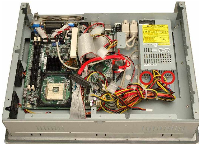
Figure 4-12: PSU Bracket Retention Screws
