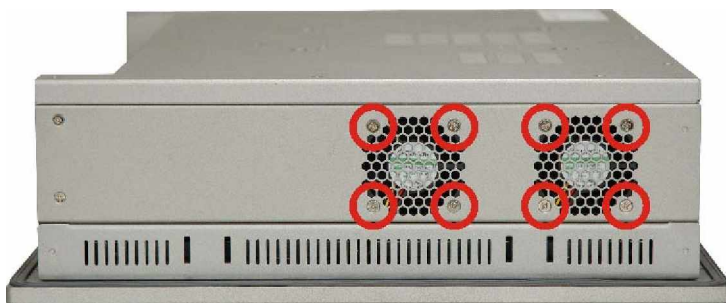
Figure 4-14: System Cooling Fans Left Panel Retention Screws
