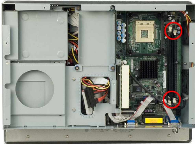
Figure 4-8: DIMM Socket Clip Locations
