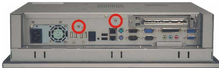
Figure 4-6: Elevated Platform Retention Screws (Bottom Panel)
