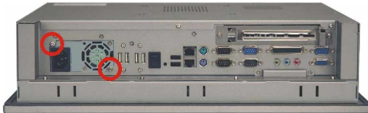
Figure 4-10: PSU Bottom Panel Retention Screws
