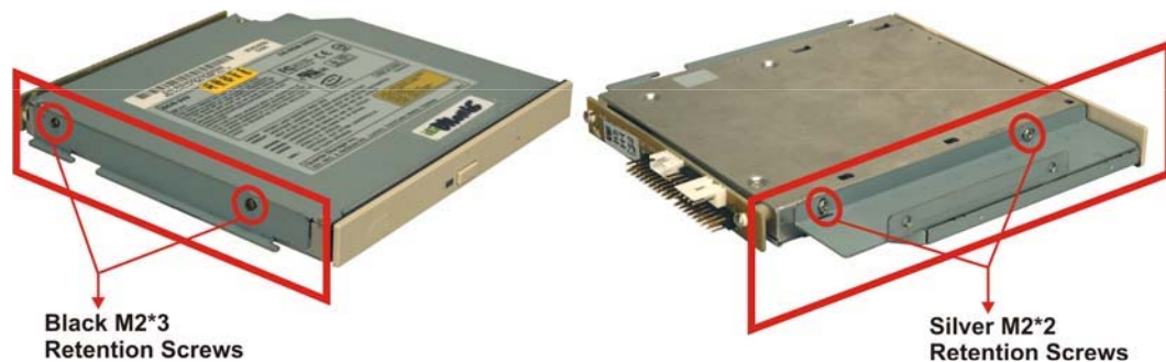
Figure 3-9: CD Drive Blank Plate Assembly
