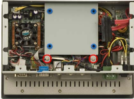
Figure 3-11: 2901230 HDD Bracket Retention Screws (Inside)
