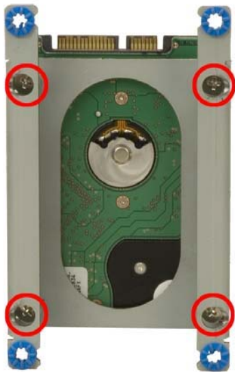
Figure 3-14: 2901240 HDD Retention Screws
