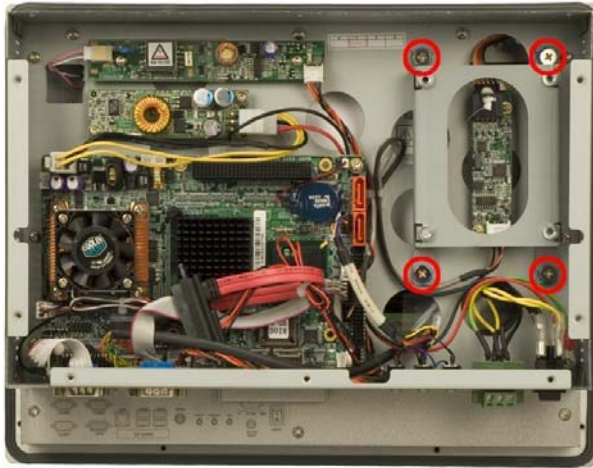
Figure 3-13: 2901240 HDD Bracket Retention Screws
