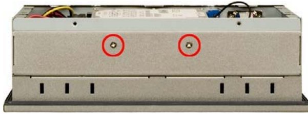
Figure 3-10: 2901230 HDD Bracket Retention Screws (Top Panel)
