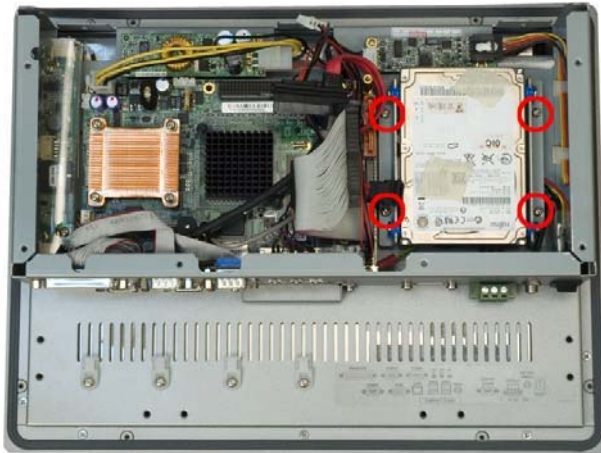
Figure 3-16: 2901250 HDD Retention Screws
