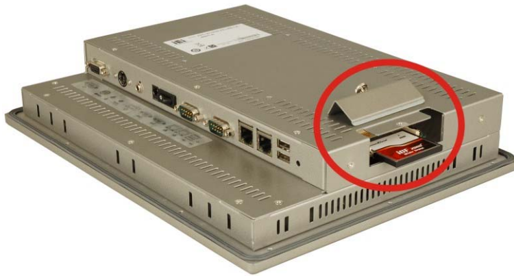
Figure 3-1: CF Card Installation
