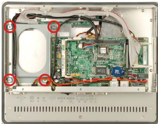
Figure 3-4: HDD Bracket Retention Screws
