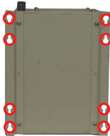
Figure 13: Locations of the 8 Wall Mounting Holes
