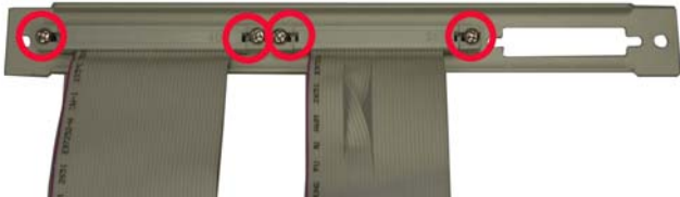
Figure 12: I/O Interface Connectors Retention Screws
