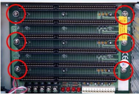
Figure 5: Insert 6 Backplane Retention Screws
