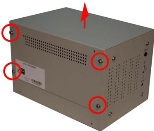
Figure 2: Remove the 8 Top Cover Retention Screws and Lift the Top Cover Up
