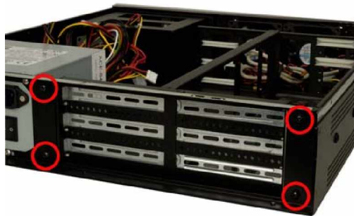
Figure 6: Four Backplane Bracket Retention Screws at the Rear of the Chassis
