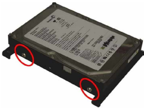
Figure 12: Insert HDD Retention Screws
