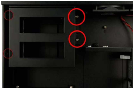
Figure 13: Four Main Drive Bracket Retention Screws
