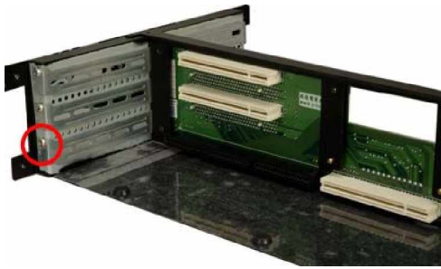
Figure 9: Remove the Slot Cover Retention Screw
