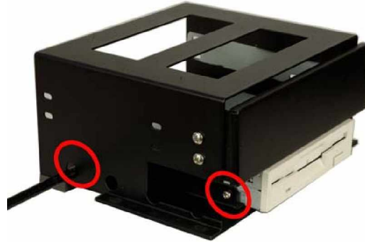
Figure 15: Insert Four Retention Screws into FDD
