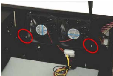
Figure 19: Remove the Two Fan Bracket Retention Screws on the Base of the Chassis
