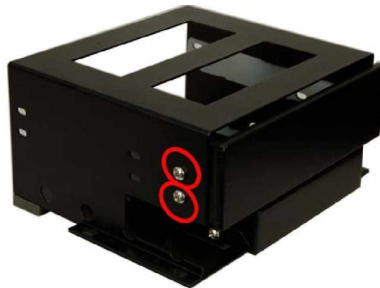
Figure 16: 5.25" Optical Drive Bay Front Cover Retention Screws
