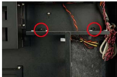
Figure 5: Two Backplane Bracket Retention Screws on the Base of the Chassis
