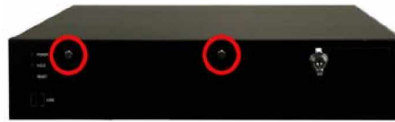
Figure 21: Loosen the Two Thumbscrews on Fan Filter Cover
