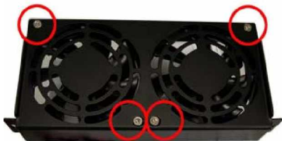
Figure 20: Locations of Fan Retention Screws
