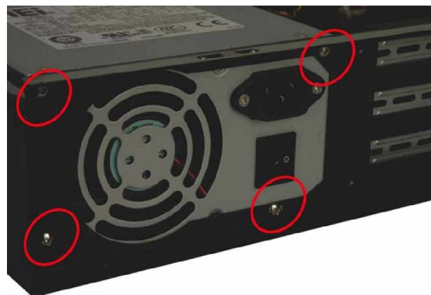
Figure 4: Insert Four PSU Retention Screws
