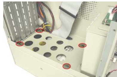
Figure 13: Elevated Predrilled Screw Holes
