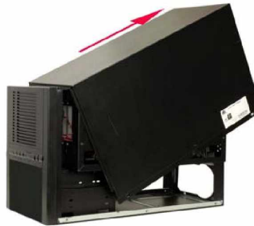
Figure 3: Remove the Top Cover
